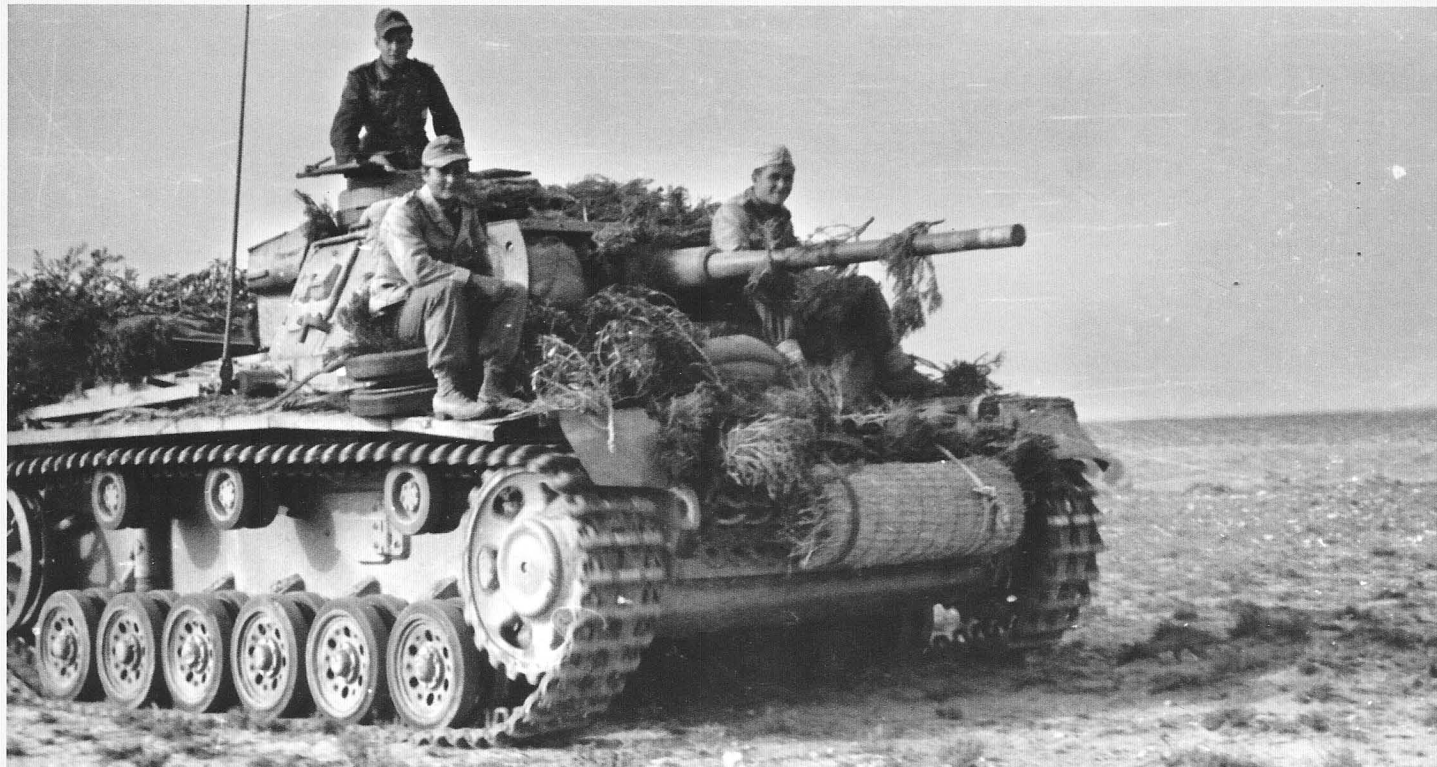
Above and left: Two views of the same Pzkw III lang. Sandbags have been fitted in front of the gun shield to replace the missing 20mm plate. The face hardened plates were particularly effective against earlier types of Allied anti-tank shells, breaking their tips before they could penetrate the main armour plates. Bottom left: A rear view of the same 8-cwt lorry seen on page 23. The letters FP probably stand for Feld Post - the number was allocated to a unit for security reasons allowing the mail to be forwarded without disclosing the unit location. Bottom right: A short barrelled Pzkw III. Markings were either few or covered by stowage. (NARA)
