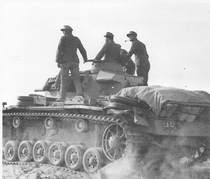
Above and left: Two views of the same Pzkw III lang. Sandbags have been fitted in front of the gun shield to replace the missing 20mm plate. The face hardened plates were particularly effective against earlier types of Allied anti-tank shells, breaking their tips before they could penetrate the main armour plates. Bottom left: A rear view of the same 8-cwt lorry seen on page 23. The letters FP probably stand for Feld Post - the number was allocated to a unit for security reasons allowing the mail to be forwarded without disclosing the unit location. Bottom right: A short barrelled Pzkw III. Markings were either few or covered by stowage. (NARA)
