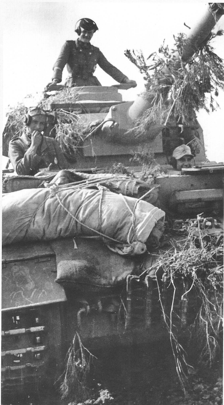
The Pzkw IVs were closely followed by two Pzkw III Ausf Ns. The second seems to have been painted in a two colour camouflage scheme. The prescribed colours at this time were of a base coat of RAL 8020 with disruptive pattern of RAL 7027. The latter colour was to be applied with a spray gun - the edges to be feathered - and was to cover approximately 1/3 of the surface area. (NARA)
