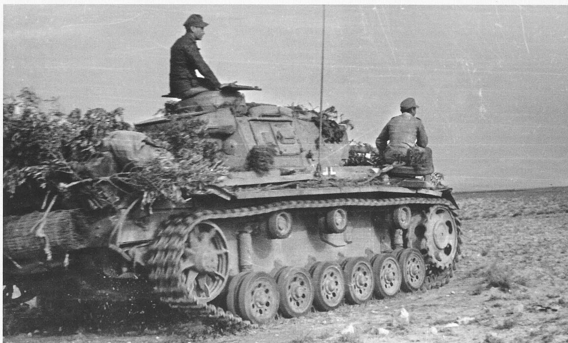
Above and left: Two views of the same Pzkw III lang. Sandbags have been fitted in front of the gun shield to replace the missing 20mm plate. The face hardened plates were particularly effective against earlier types of Allied anti-tank shells, breaking their tips before they could penetrate the main armour plates. Bottom left: A rear view of the same 8-cwt lorry seen on page 23. The letters FP probably stand for Feld Post - the number was allocated to a unit for security reasons allowing the mail to be forwarded without disclosing the unit location. Bottom right: A short barrelled Pzkw III. Markings were either few or covered by stowage. (NARA)
