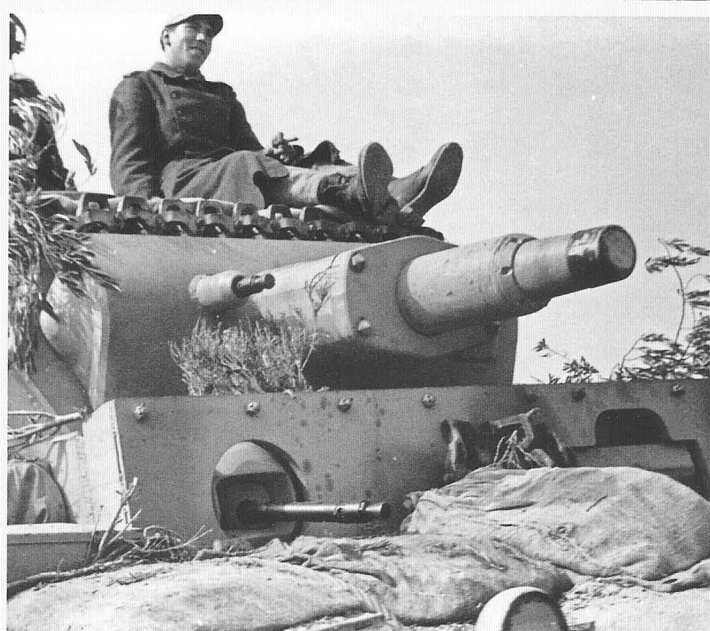
The Pzkw IVs were closely followed by two Pzkw III Ausf Ns. The second seems to have been painted in a two colour camouflage scheme. The prescribed colours at this time were of a base coat of RAL 8020 with disruptive pattern of RAL 7027. The latter colour was to be applied with a spray gun - the edges to be feathered - and was to cover approximately 1/3 of the surface area. (NARA)
